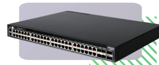
AS4610-54T 48 x 1G Base-T 4 x 10G SFP+ uplink ports 2 x 20G QSFP+ stacking ports
